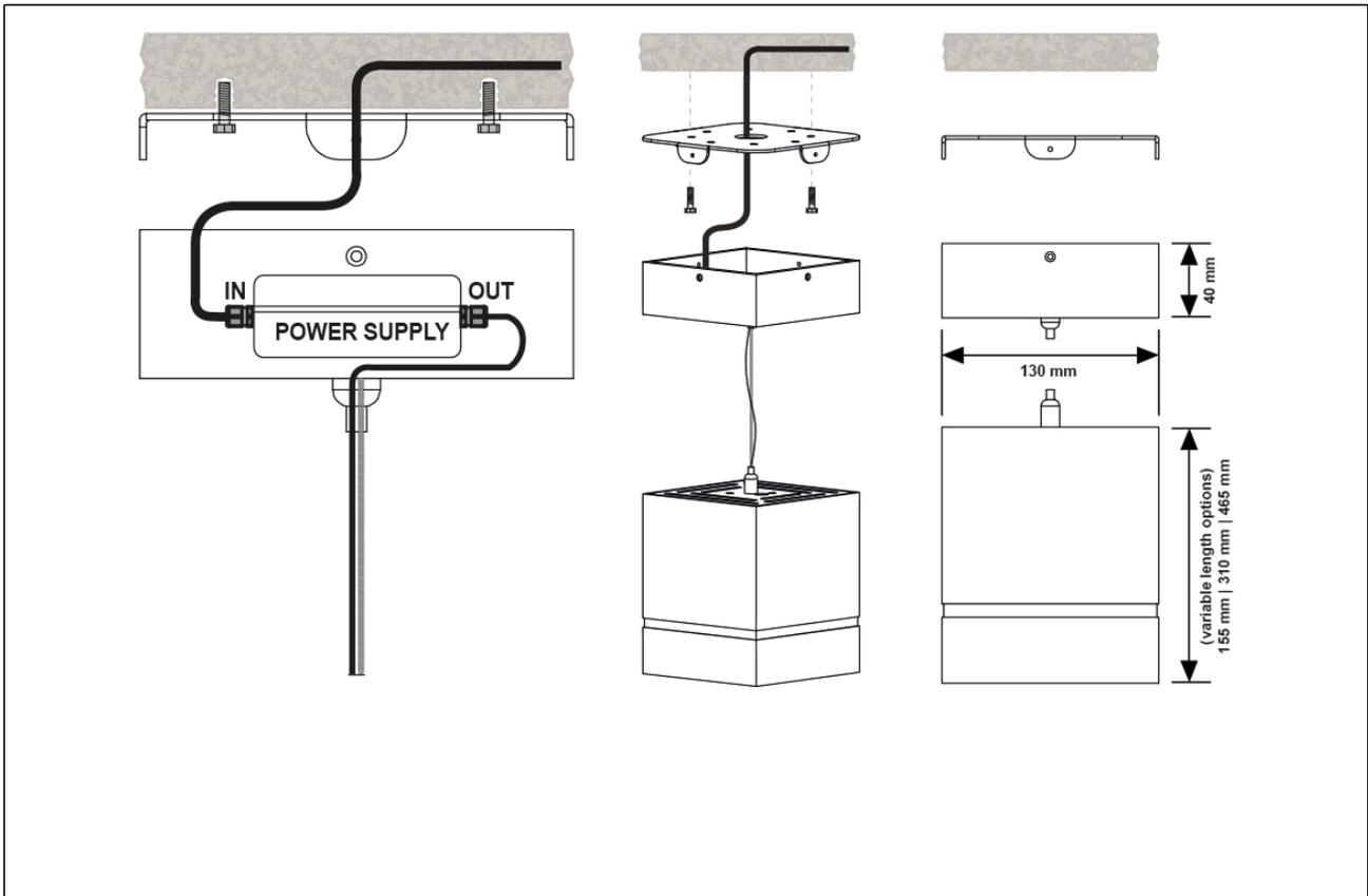
Install the provided plate and adjust like the favored direction. Use the provided cable clamps to join the wires. Install the fixture with provided screws on the plate. Assure you have tightened all screws and check again.
